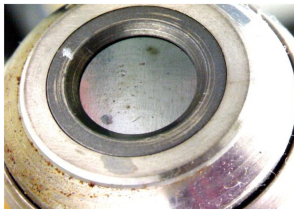
Fig. 7. Contamination and corrosion of the detector window ( 10 \text{ mm}^2 ).
